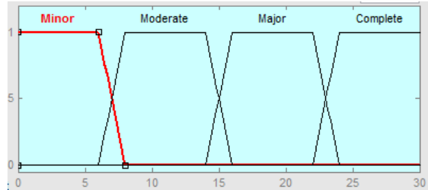
Fig. 15. Membership function shut-down command–gas–Rey fault
